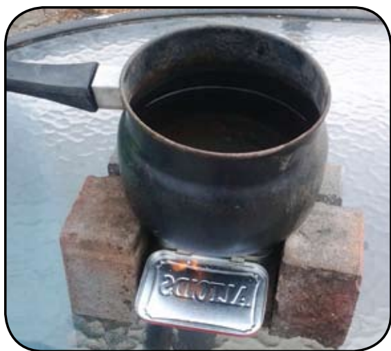
Once your bricks are layered insert the perlite-filled Altoids container.
